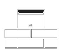
Build up brickwork to desired height and set letterbox in place
