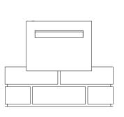
Build up brickwork to desired height and set letterbox in place
