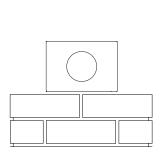
Build up brick work to desired height and set paper ring in place
