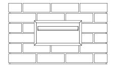
SLEEVE FITS INTO 1.5 BRICK WIDE BY 2 BRICK HIGH CAVITY Build up brickwork to desired height and set letterbox in place
