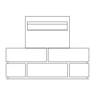
Build up brickwork to desired height and set letterbox in place
