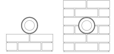
Build up brick work to desired height and set paper ring in place
