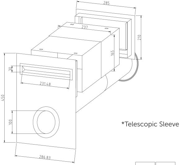
NOTE: MEASURE THE DISTANCE FROM SLEEVE TO RING IN ORDER TO FIT SLEEVE INTO NORMAL BRICK COURSE
