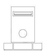
Build up brickwork to desired height and set mail tube in place
