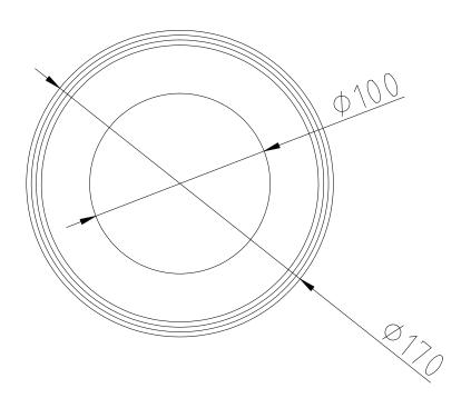
Cut a piece of 100mm PVC Pipe to the desired length. Slide the PVC pipe over the paper ring. Secure and seal with silicone or similar adhesive.
