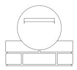
1.Build up brickwork to desired height and set letterbox in place
