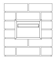
SLEEVE FITS INTO 1 BRICK WIDE BY 2 BRICK HIGH CAVITY Build up brickwork to desired height and set letterbox in place
