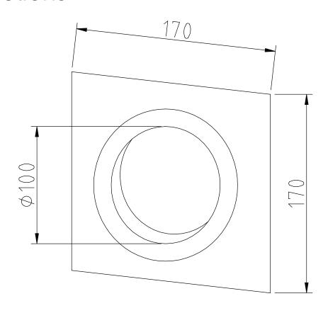
Cut a piece of 100mm PVC Pipe to the desired length. Slide the PVC pipe over the paper ring. Secure and seal with silicone or similar adhesive.
