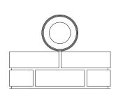
Build up brick work to desired height and set paper ring in place
