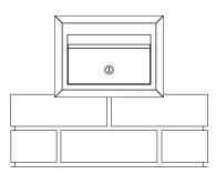
Build up brickwork to desired height and set letterbox in place
